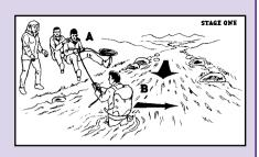
holds the rope, which has a knot in the end to increase grip. An overhand knot is ideal but the loop formed should be small so that a hand cannot pass through it and risk entanglement.
